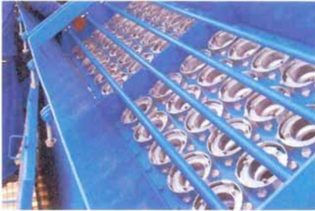
Multiple filter bag housings shown within one of the four plenum chambers located on all sides of the 7.5 m square hopper inlet.
