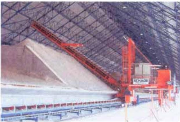
A Schade cantilevered boom reclaimer recovering additives from segregated stockpiles.
