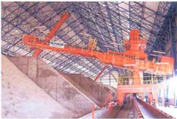
Schade travelling and luffing boom stacker stockpiling additives and gypsum to segregated storage areas.
