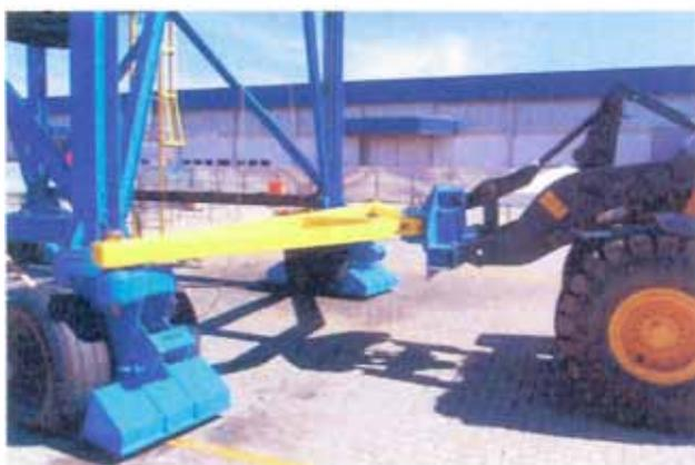
Eco-Hopper with towing tractor and 'Ackermann' linkage to steering wheels with integral supporting jacks to take the operational load.
