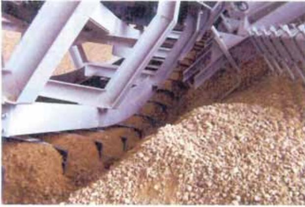
The Schade chain scraper conveyor shovels collect the limestone from the reciprocating harrow and raise it to the collecting conveyor running parallel to the stockpile.
