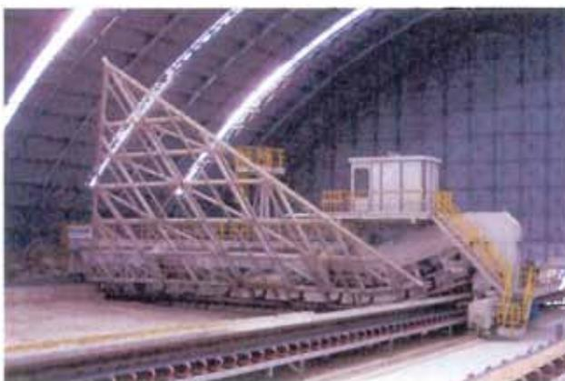
Schade bridge reclaimer with single sided reciprocating harrow for recovery and blending of limestone from a single stockpile.
