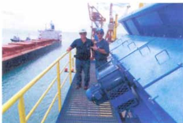
One of four Eco-Hopper dust filter units positioned along each side of the grab hopper inlet; Panamax vessel berthing in the background.
