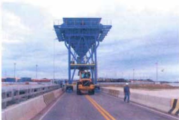
Mobile Eco-Hopper with mobile harbour crane imports clinker and slag from 70 000 t gearless Panamax bulk carrier.
